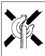
Fig 2 c Hook latch obstructed
