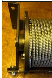
Fig 3 U-bolt secures rope
