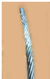
Fig 1 Secured rope end
