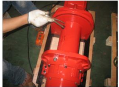
Fig 10 Fixing the wire rope to the drum.
