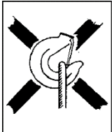
Fig 3 a The sling is applying load to the hook tip
