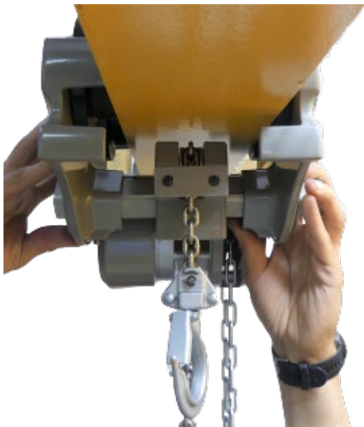
Pic. 2 Raise the Smart Hoist and slide both side plates against the lower flange of the beam
