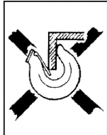
Fig 3 d Hook tip subject to additional bending stress
