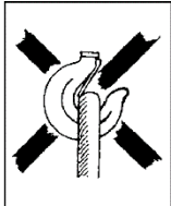
Fig 3 c Hook latch obstructed
